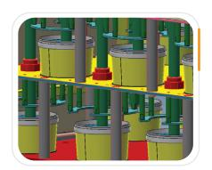
The High Viscosity module can handle up to 20 components and it is fitted with a specially designed press-out mechanism c/w press pumps equipped with rubber follower plates. The module is engineered to store the inks n their original packaging, 2.5, 3 and 5 kg plastic or metal cans.
